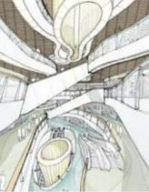
We wanted the mall to feel bright and airy, so included a series of voids penetrating the building. These spectacular spaces are spanned by circulation 'bridges' to help with visitor flow, while sunken 'pools' feature at ground level, creating seating areas.
